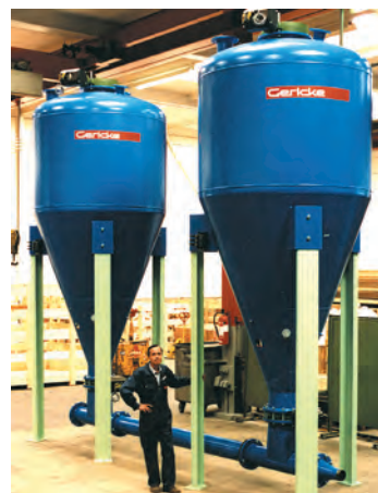
Continuous conveying of fly ash at 130 m 3 /h with double sender.
