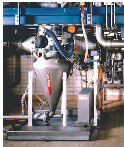
Chemical products: Pneumatic dense phase conveying with weighing and throughput recording.
