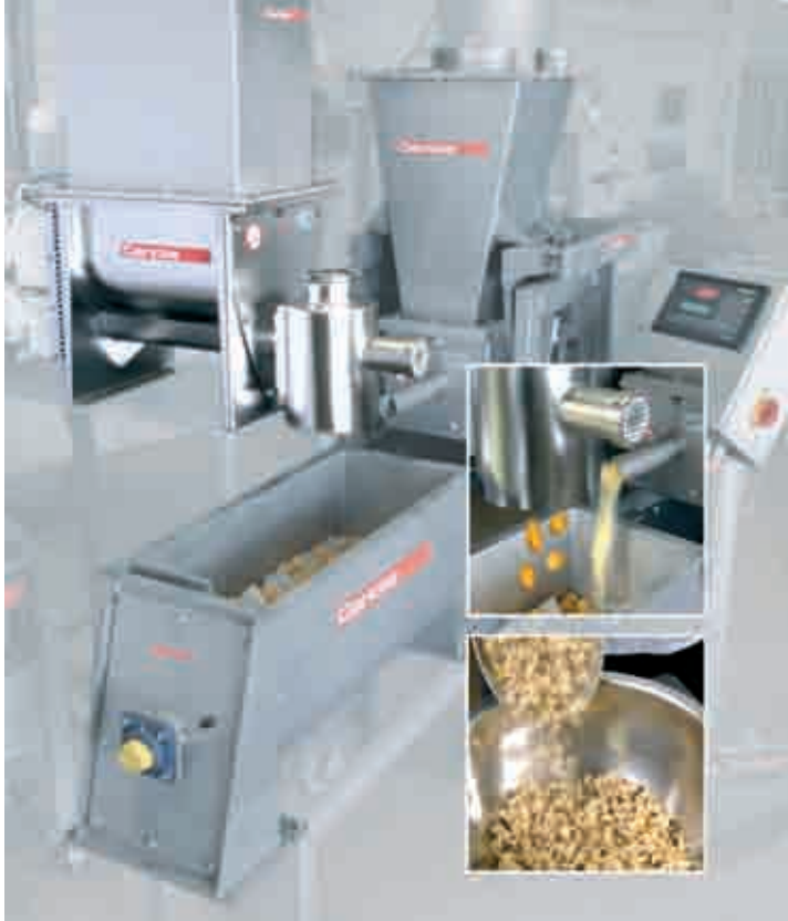
Controlled feed into a Gericke continuous mixer
